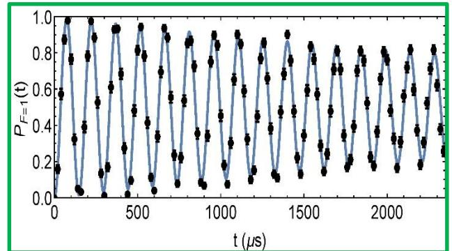
Fluctuations in the magnetic field causes dephasing
