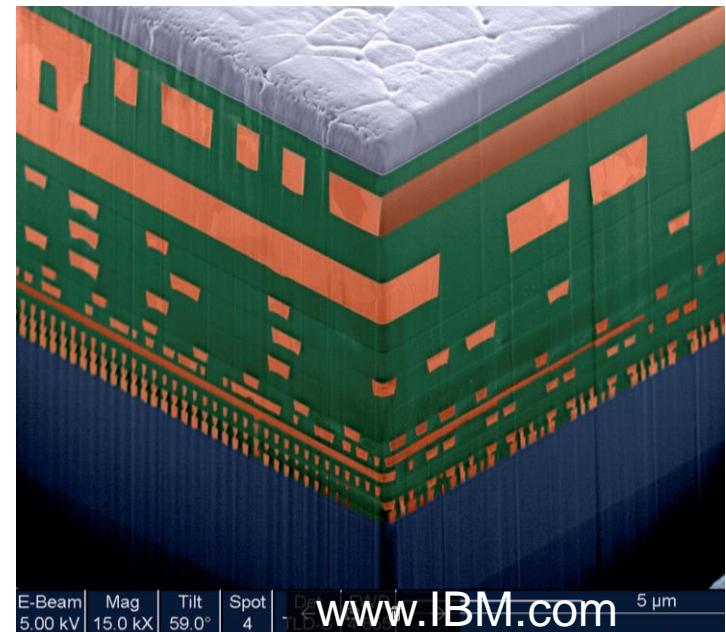
IBM microprocessor chip:
