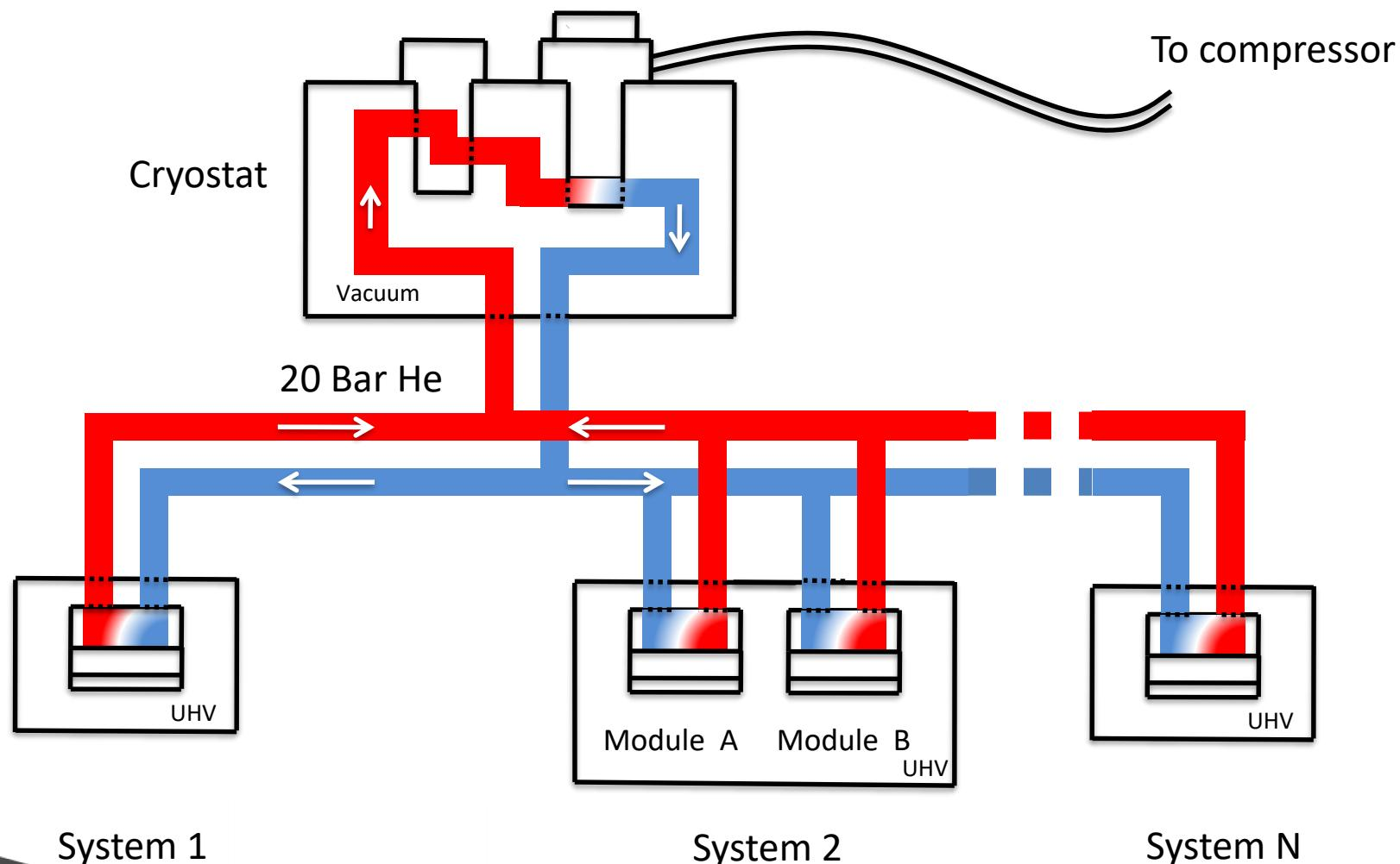
Cooling system is required to cool relevant classical electronics
